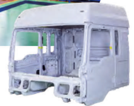
▲ Cab remanufactured product of MAN Tractor
